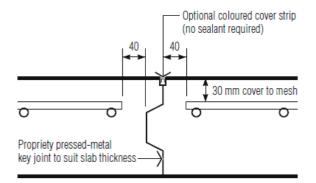
(b) KEY JOINT (PRESSED-METAL OR FORMED)
