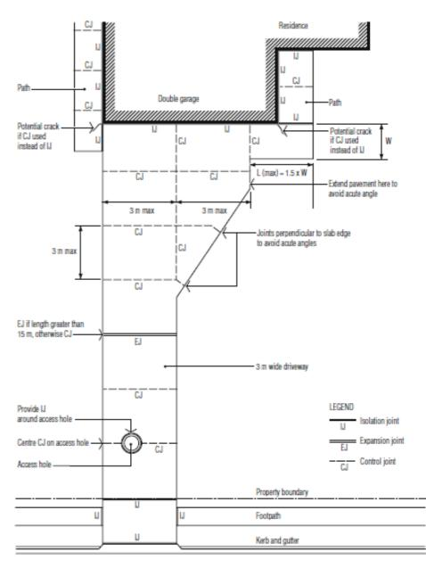
Figure 2: Typical joint layout
