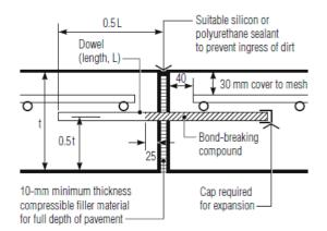
Figure 6: Typical expansion joint
