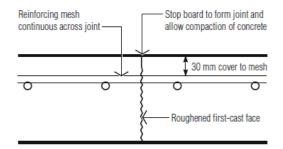
Figure 8: Typical construction joint
